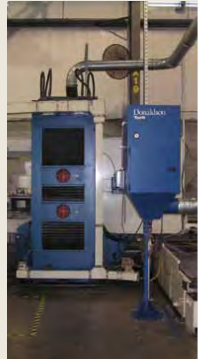
WSO Horizontal grinder 850 cfm
